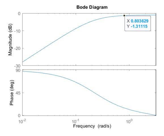
In the figure above, we have a Bode plot for the backward Euler. We can see that at omega = 0.80, the frequency response turns flat.
