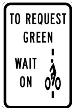
■ FIGURE 2-7 Bicycle detection in Phoenix
